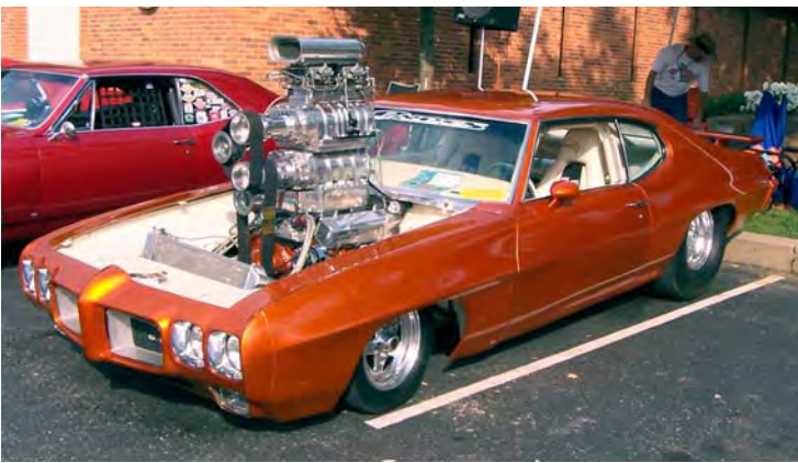
Up periscope! Subtle modifications to Bill Bolin's '70 GTO include 8-71 blower mounted atop 6-71 blower, full custom interior, and eye-catching orange paint.
